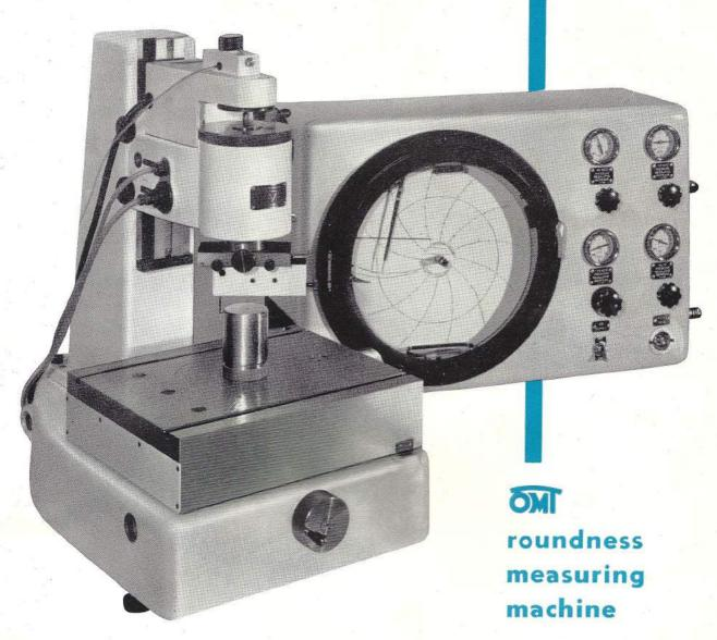
Providing facilities for roundness measurement to an extremely high order of precision, this equipment, developed in conjunction with the National Engineering Laboratory, East Kilbride, is offered at a price permitting it to be considered for general workshop application and production line inspection in addition to standards room employment.
