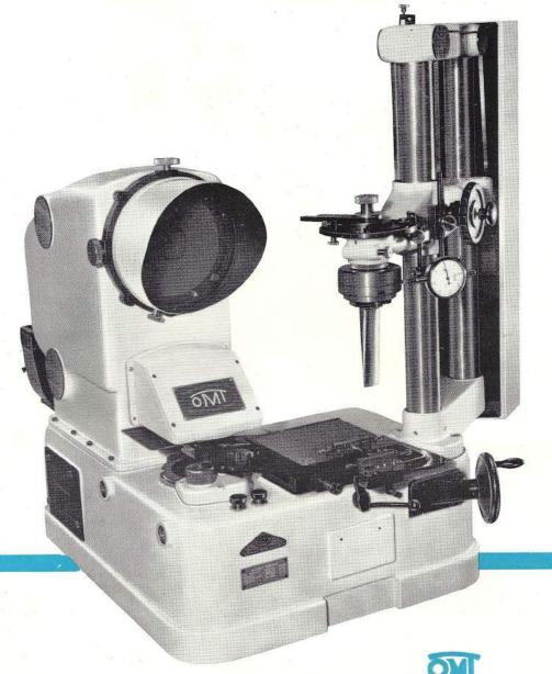
This instrument has been developed for the rapid and accurate inspection of three dimensional contours, such as turbine blades, where the normal method of projection is impossible due to the interference in the light beam of the twist in the blade or the root. By means of an optical system a magnification of 30x is used with a screen of 6" diameter and blades of 3" wide by  $15\frac{1}{6}$ " long can be inspected for size, accuracy of radii, thickness at various positions
