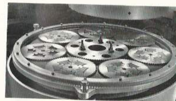
Detail of the geared workholder designed for the above machine in order to ensure full and constant rotation of the workholder.
