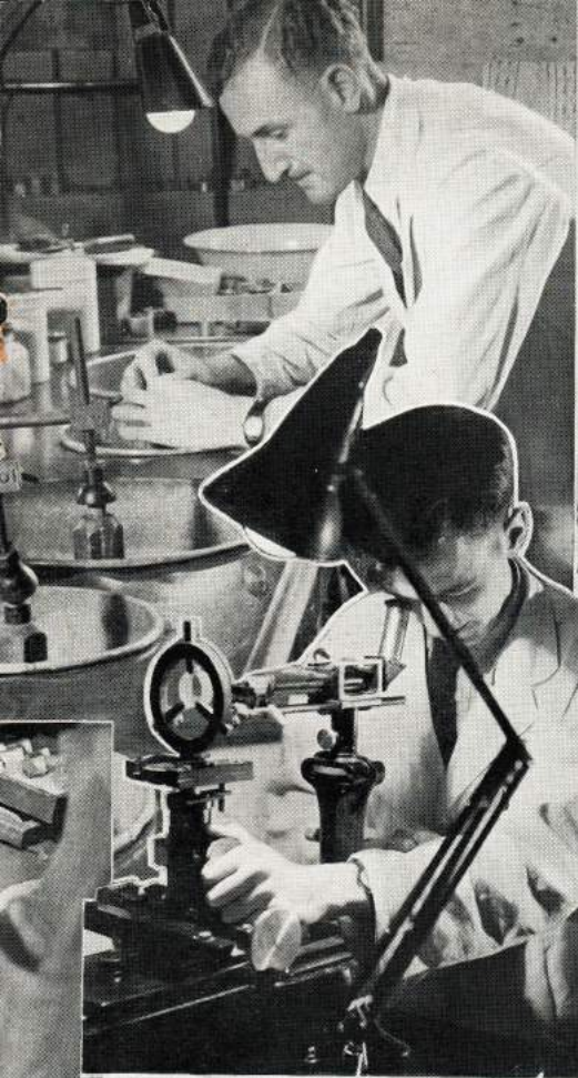
(Above) A lense being checked for definition and perfect sphericity. (Right) A view showing a vacuum pump and chamber used for the "blooming" of lenses, also for the illuminising of mirrors.
