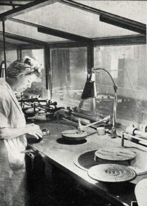
(Above) View of optical machines with dust-proof covering, showing prisms in course of examination and polishing. (Below) Toolmakers' microscope being assembled and inspected.
