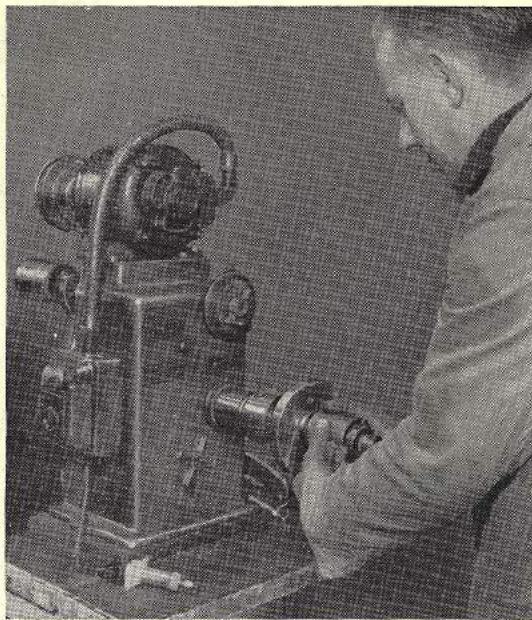
8 Any errors in roundness or parallelism are corrected by lapping the pivot with a cast-iron split lap, charged with diamond compound
