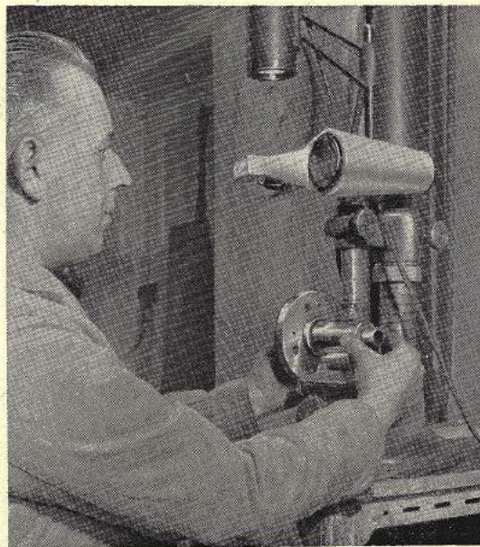
7 Checking the diameter of a pivot with the aid of an OMT vertical Omtimeter, prior to the lapping operation
