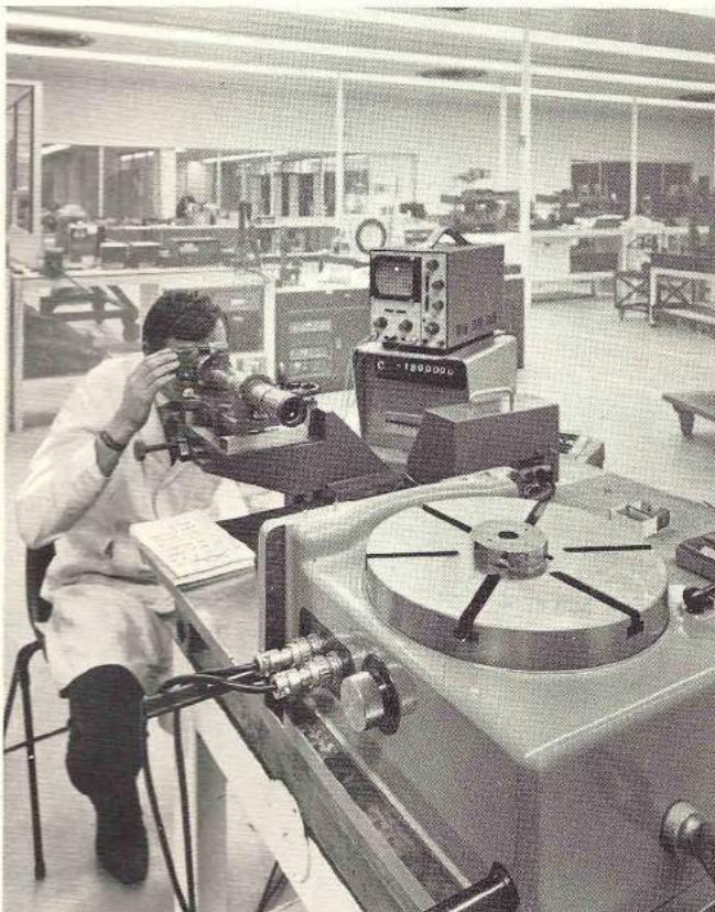
Testing of a rotary indexing table with the aid of an autocollimator, polygon and oscilloscope.
