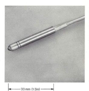
A need which now had to be met was for a miniature measuring probe for close proximity gauging. Q.C.S. Development Engineers succeeded in producing a miniature probe (4) so small, yet so accurate, that even in pairs discrimination to two hundred and fifty millionths of a millimetre (ten millionths of an inch) could be achieved.
