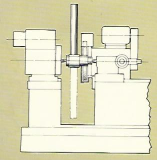
The Butler Newall Gap Bed Grinder (GBG) has been specifically designed to accommodate components which would be impractical to grind on any conventional machine.
