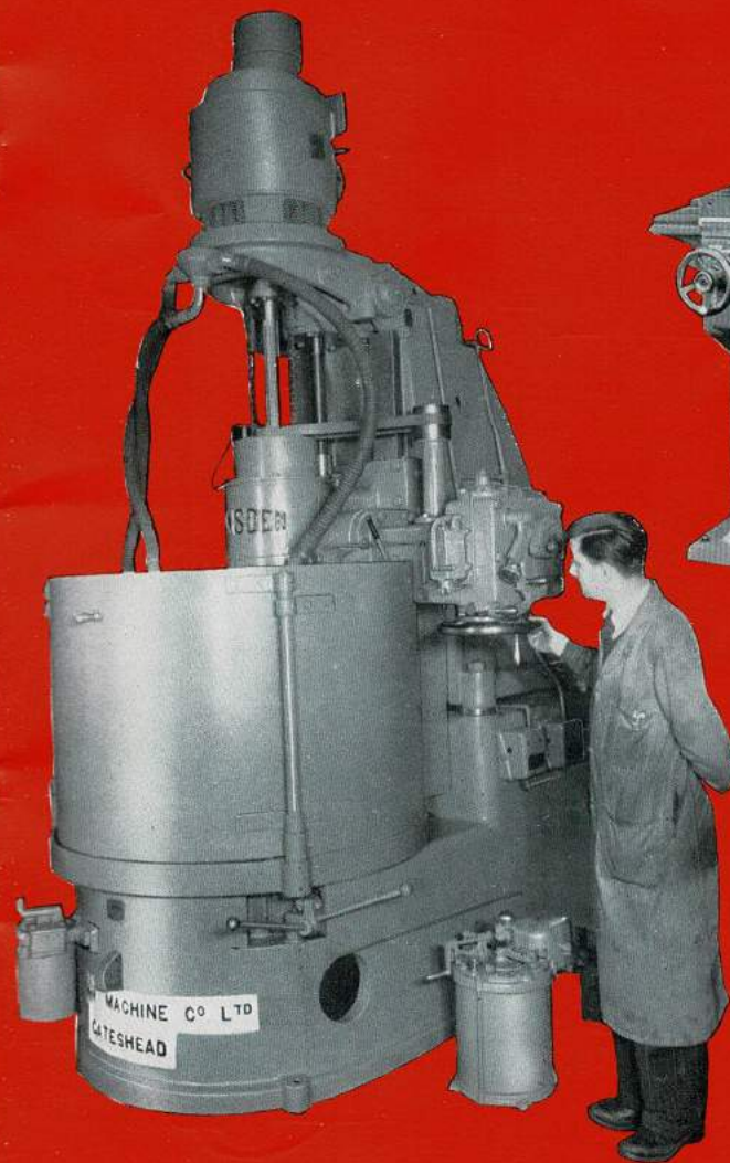
Below : This Lumsden surface grinder illustrates the diverse range of machines re-precisioned by Newall.
