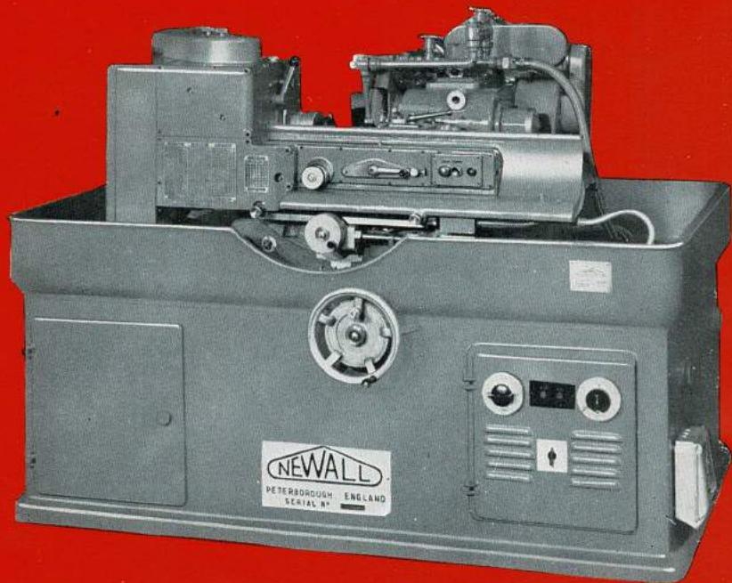
Top : Newall model 420 thread grinder re-precisioned for tool-room and production use.
