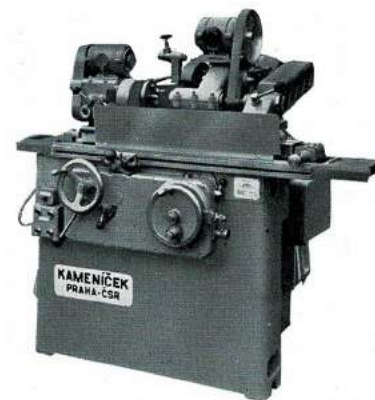
A Kamenicek universal grinder, one of many foreign products re-precisioned by Newall.
